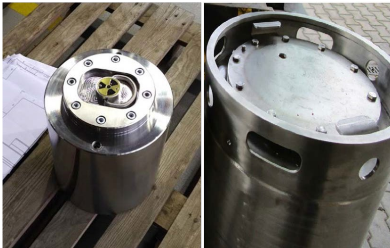
Figure 4. Lu-177 and Y-90 Transportation Flask (left) and Overpack (right)
