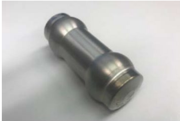
Figure 1. Exterior of Mo-99, Lu-177, and Y-90 Target Capsule
