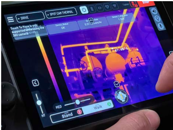
FIGURE 20 – OPERATOR VIEW OF SPOT THERMAL IMAGING CAMERA
