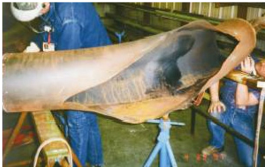
Failure in a high pressure extraction line at Fort Calhoun in 1997
