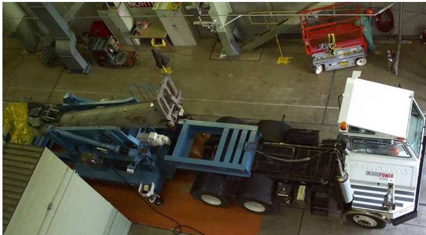
Transporter/Erector and truck at Pickering NGS
