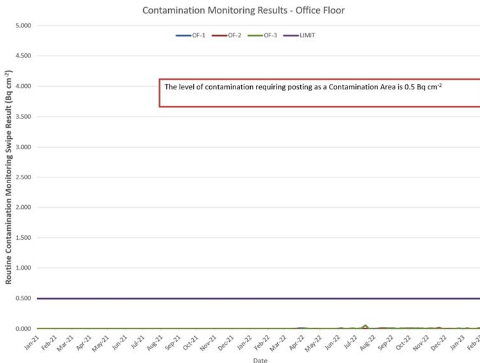
Figure 2.7.2-5 – Contamination monitoring results for the office floor
