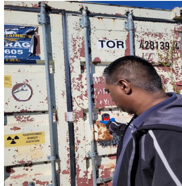
CNSC inspector verifies dose rate readings around trailer containing waste (source: CNSC staff)
