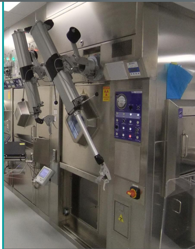
Hot cells used for handling unsealed nuclear substances produced in a cyclotron (source: CNSC staff)
