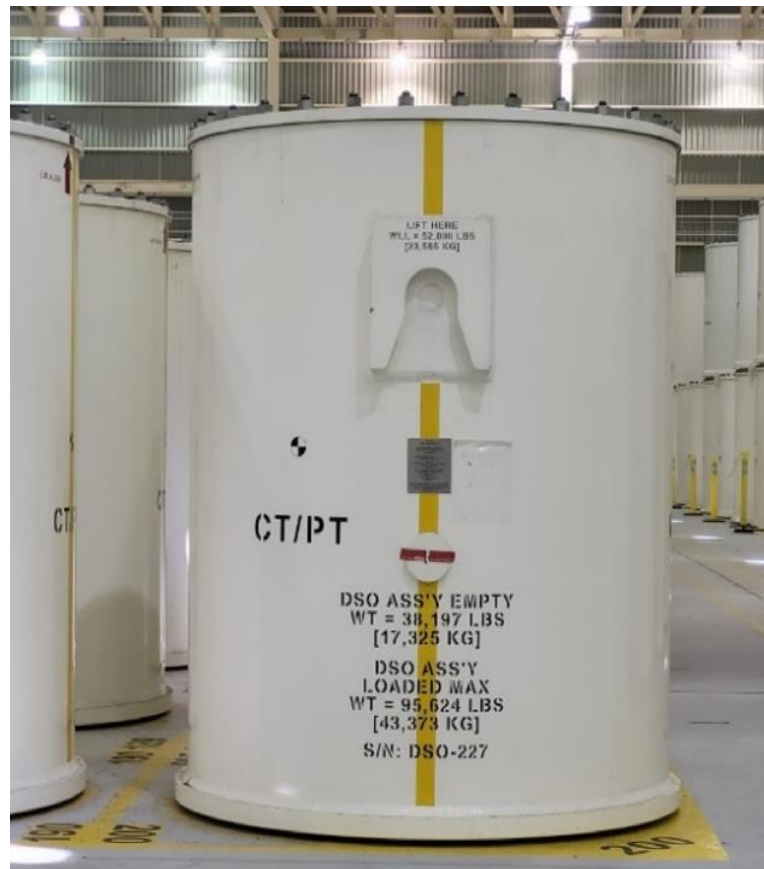
Figure 3: Darlington Storage Overpack with Retube Waste Container inside Source: Ontario Power Generation
