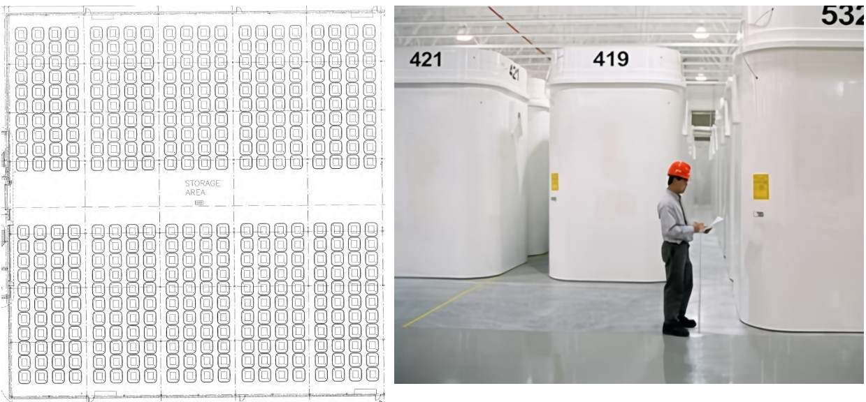
Figure 7 : Storage Plan of OPG NWMF building # 1 (left); Store casks (right) - see how an efficient use of space to store also means you cannot remove a specific cask easily
