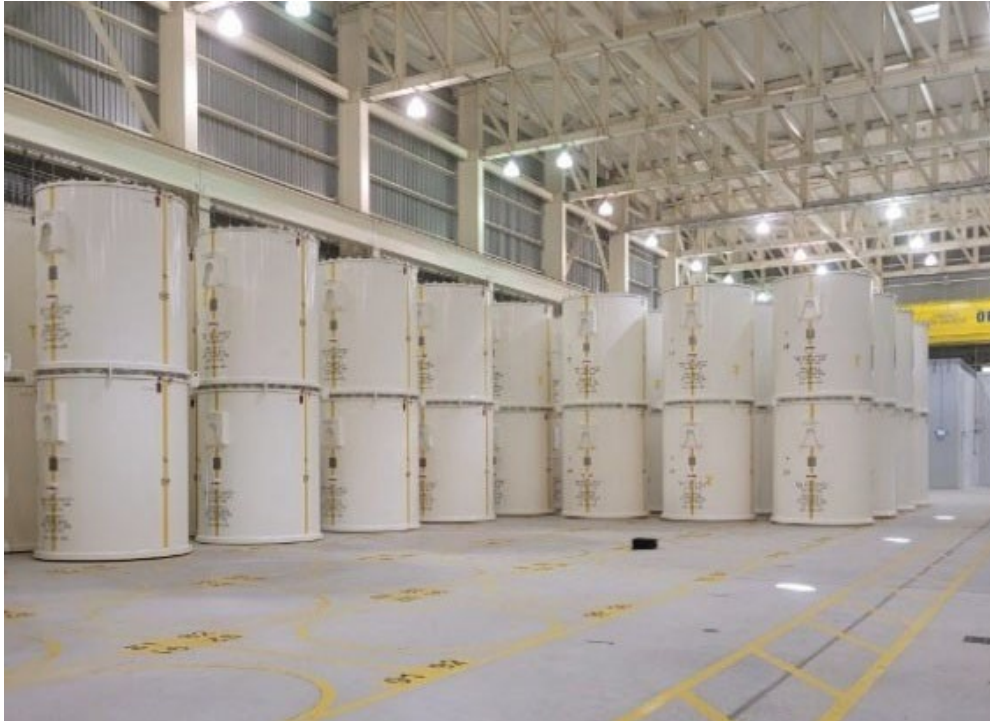
Figure 14: RWC/DSOs Stacked Two-high in the RWSB
