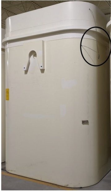
Figure 21: DSC in Storage showing IAEA Cobra Seals
