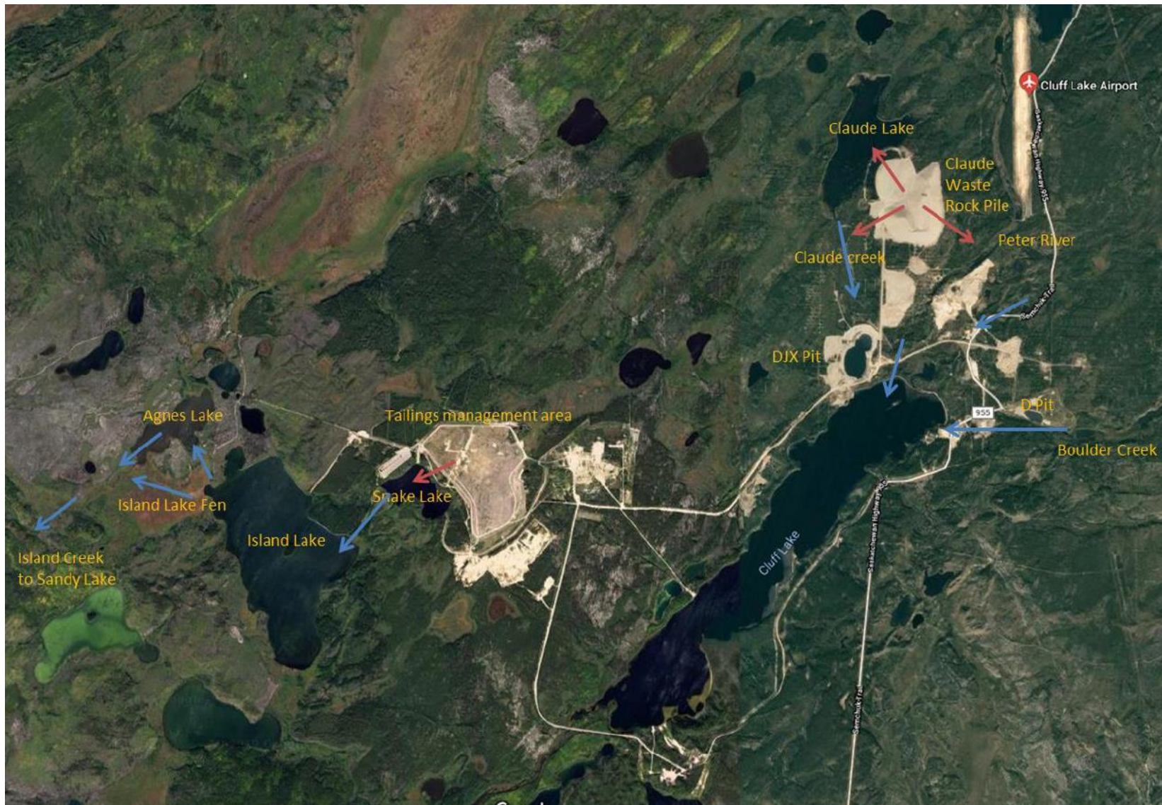
Figure 5: Drainage from mine features (red arrows) and water flow on site (blue arrows)
