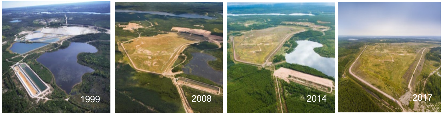
Figure 2-4: Time Series of the Tailings Management Area
