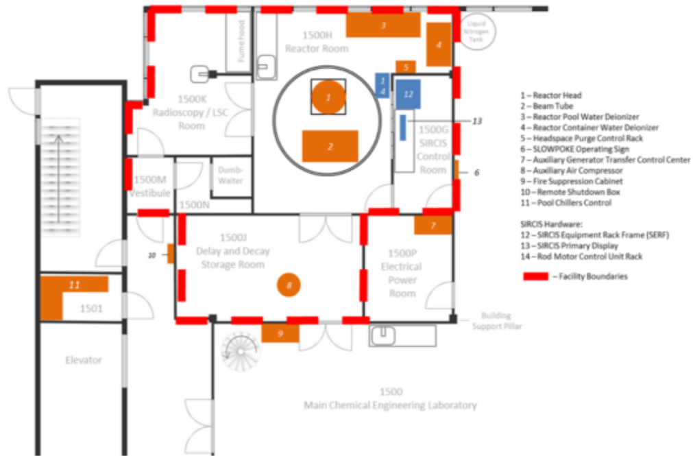
Figure 3: RMC SLOWPOKE-2 reactor location within Sawyer Building
