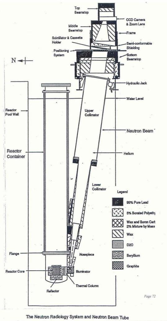
The Neutron Radiology System and Neutron Beam Tube
