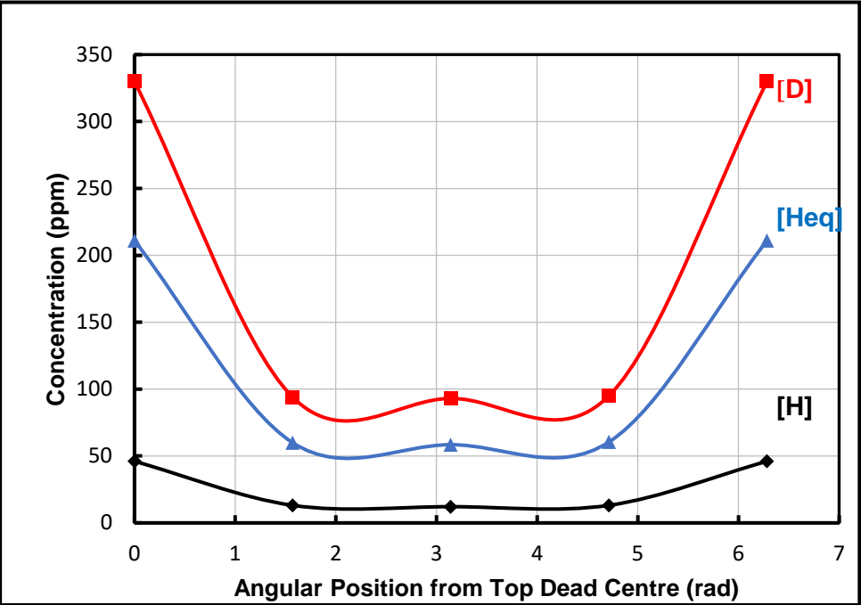
Circumferential Distribution of [H], [D], and [Heq] at the Outlet PT RJ of B6S13 at 271, 729 HH
