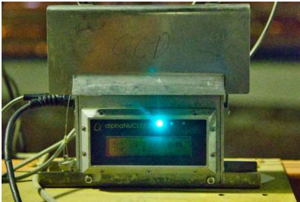
Figure 2.2: AlphaNUCLEAR PRISM at an underground mine
