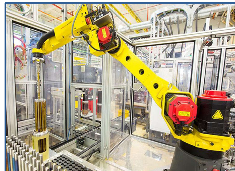
Robot inserting rods into fuel bundle assembly at Cameco Fuel Manufacturing Source: Cameco
