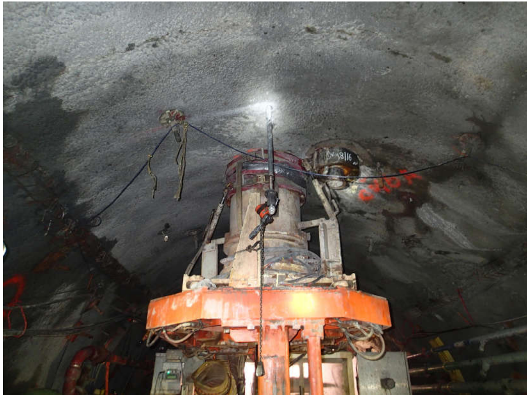
Figure 3.3: Underground jet bore used for ore removal
