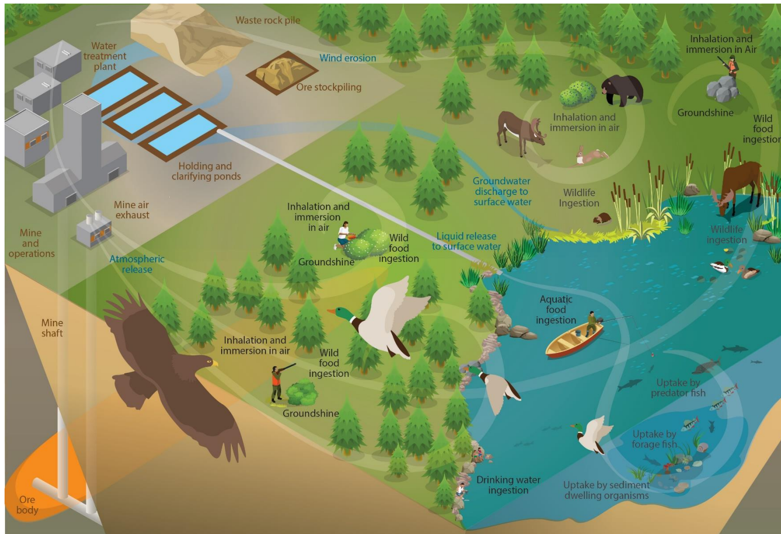
Figure 3.1. Conceptual model of a generic mine site
