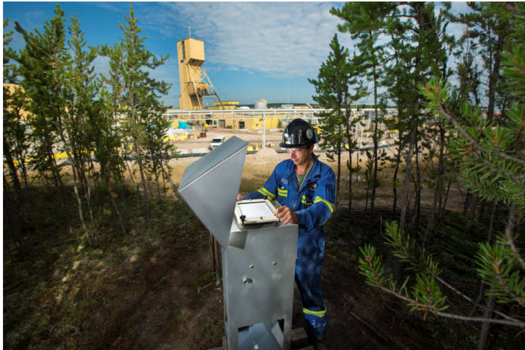
Figure 3.6: High volume air sampler at Cigar Lake
