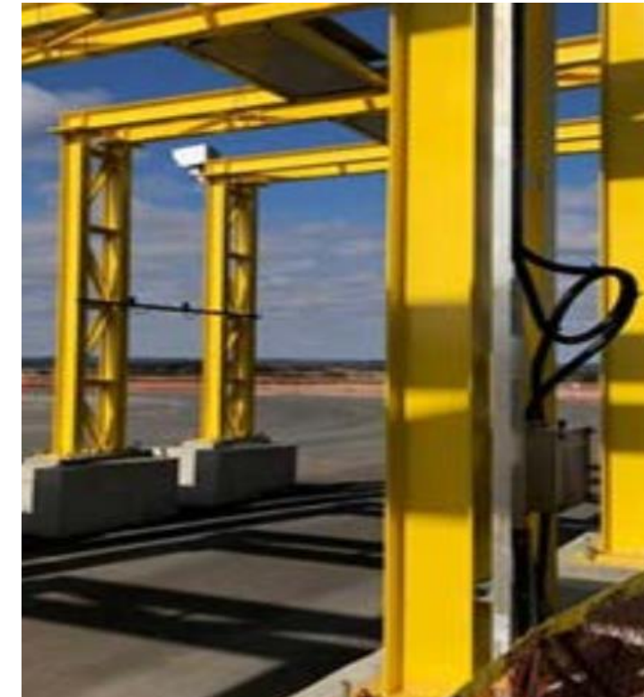
The IAEA's unattended portal monitor at the Port Hope LTWMF (courtesy IAEA)
