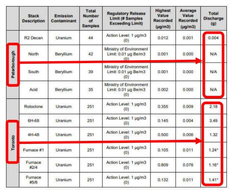
Table 18: Summary of Hazardous Substance Releases to Air at Exhaust Stack
