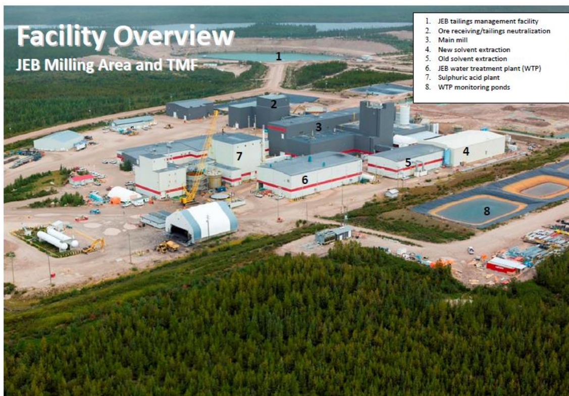
Figure 7.1: McClean Lake Operation - aerial view of the JEB milling area and tailings management facility
