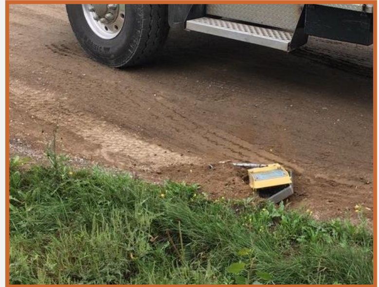
Damaged portable gauge (source: CNSC staff)
