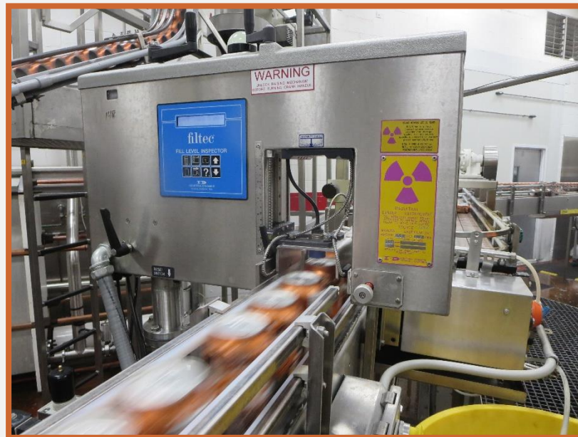
Fixed gauge measuring fill level in cans ( source: CNSC staff )
