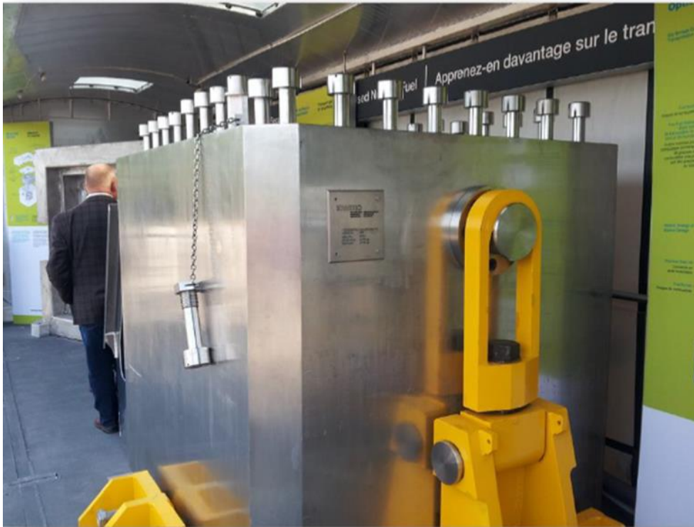
Figure 3-5: Used Fuel Transportation Package for the removal of CCSF fuel to CRL
