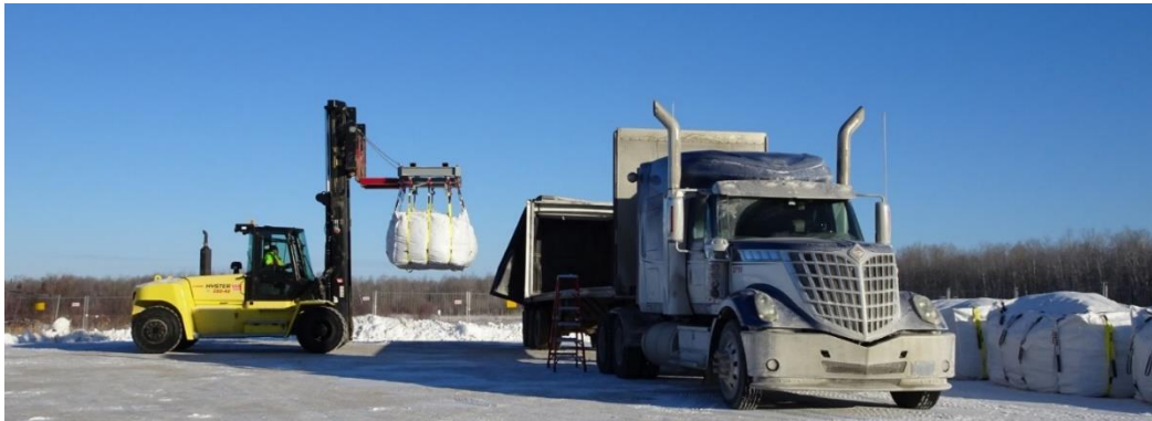
Figure 3-16 : Photo of Low Level Waste (Contaminated Cesium Pond Soil) being loaded for transportation to CRL
