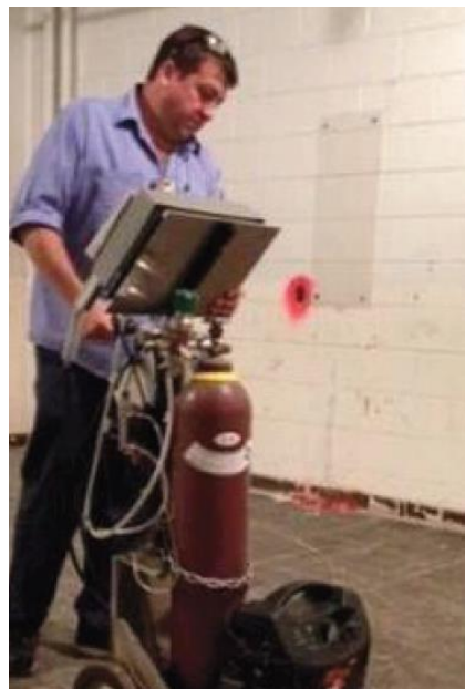
Figure 10-2 : Surveying a Decommissioned Room for Radioactive Contamination.
