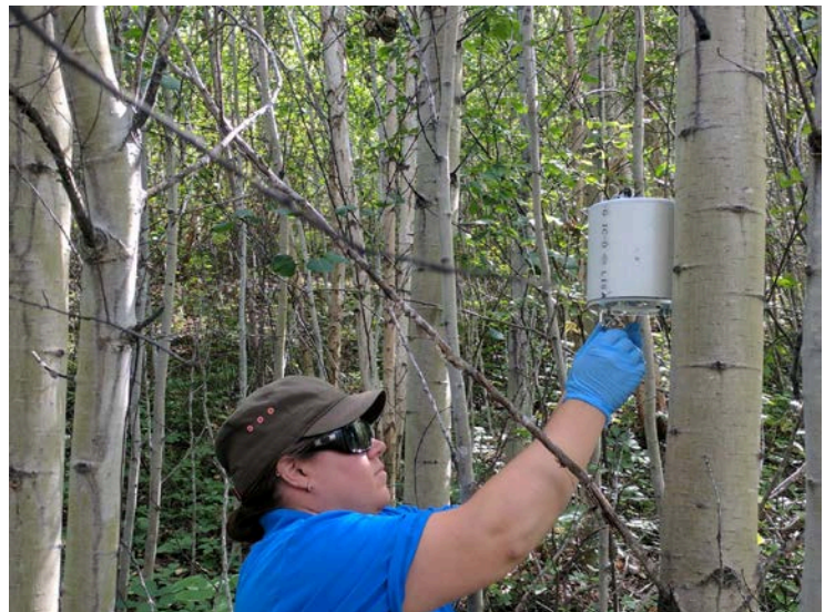
Figure 11: CNSC staff installing a radon sampler near the Cluff Lake Project site in 2017
