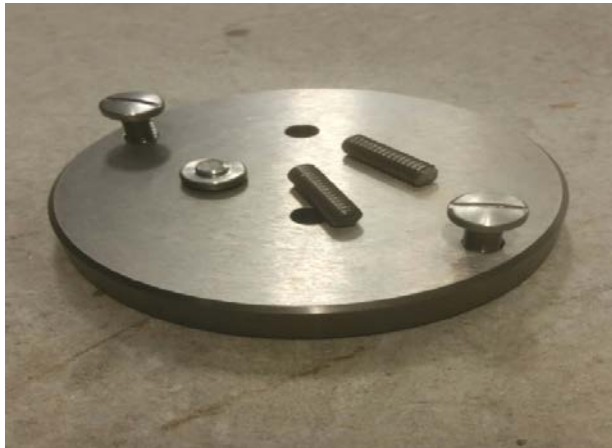
Figure 4: Broken tungsten screw and end plug
