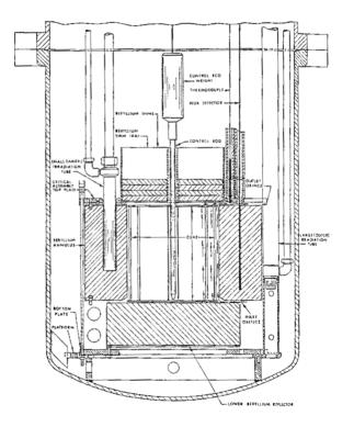
Figure D-2 Critical Assembly (Cross-Section)
