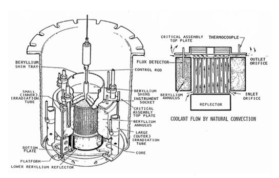
Figure D-4 Lower Reactor Container
