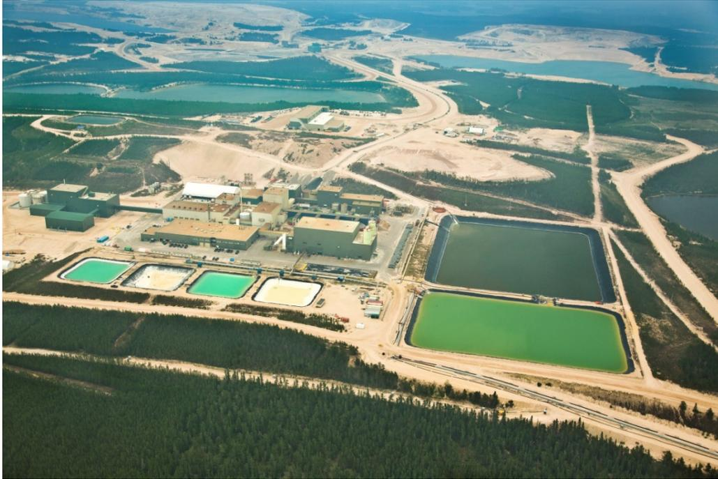
Milling of the stockpiled Deilmann ore continued until 1999, when the McArthur River Operation began supplying ore slurry to the Key Lake mill. The Key Lake Operation continues today as a mill operation processing McArthur River ore slurry and residual special waste from previous mining at Key Lake.
