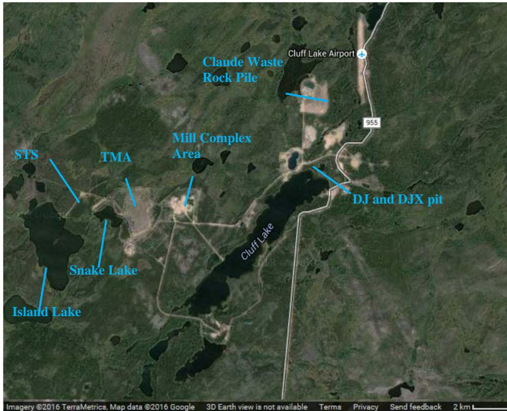
The former Cluff Lake Operation consisted of a central mill, above ground tailings management area (TMA), three open pits, two underground mines, associated waste rock piles, and site infrastructure including an airstrip and camp (figure 14.2).
