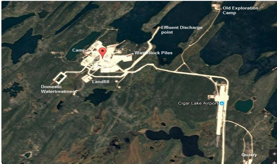
The Cigar Lake uranium deposit is mined by mass freezing the orebody and surrounding country rock. Hydraulic water jets then extract the ore as a slurry (mixture of rock and water), which is pumped to surface, loaded into containers and transported 70 kilometres by truck to AREVA's McClean Lake Operation for milling.
