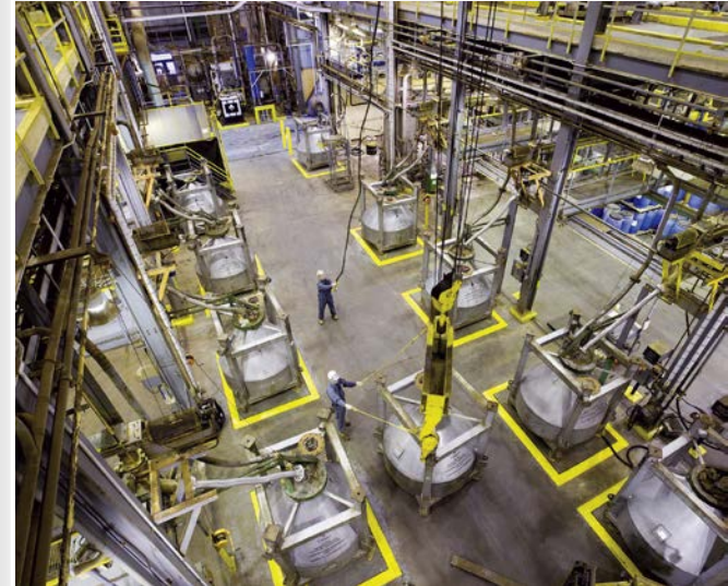
UO_3 tote bin loading and handling station at the Blind River Refinery.
