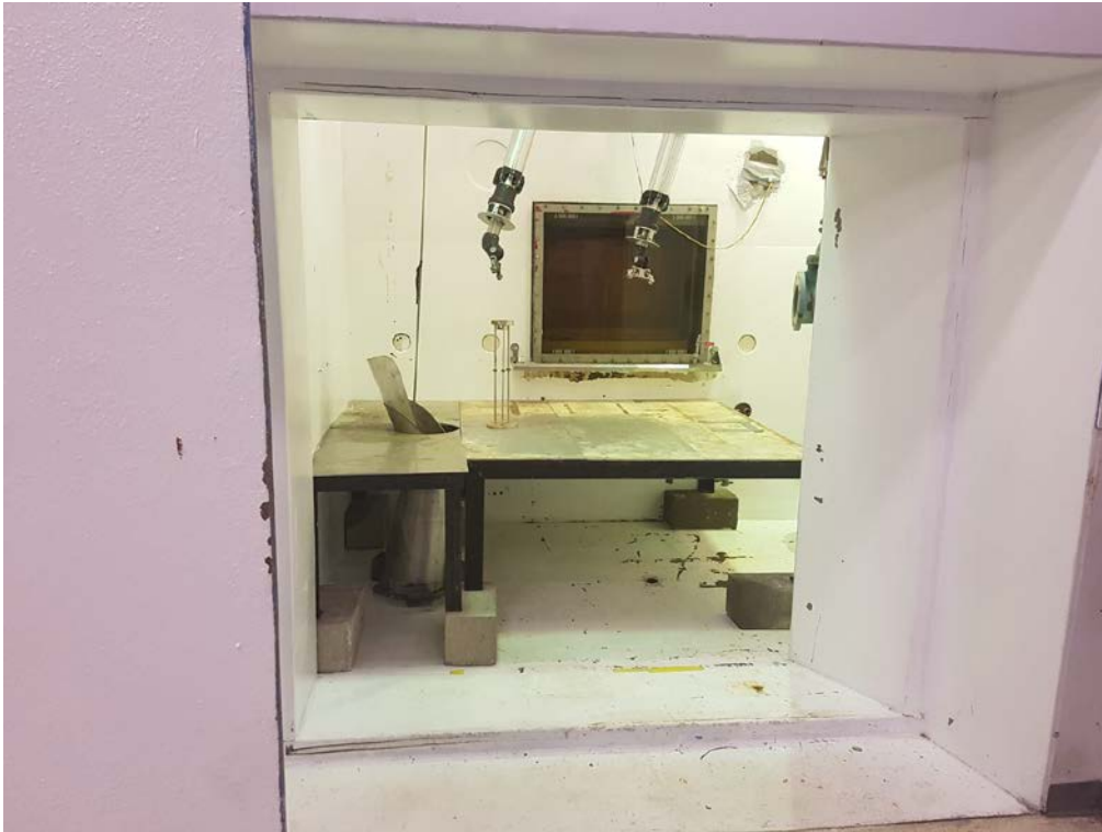
Figure 1: Interior of hot cell, viewed from service area
