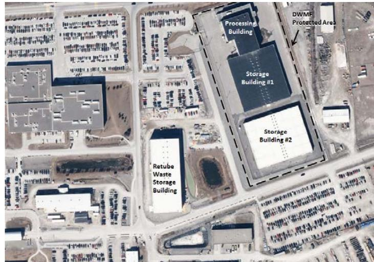
The DWMF consists of an amenities building, one DSC processing building, two DSC storage buildings (Storage Buildings #1 and #2), and the RWSB. The DWMF has the capacity to store 983 DSCs and 490 DSOs. The transfer of loaded DSCs from the DNGS to the DWMF is conducted on OPG property with a security escort and the transfer of loaded DSOs from the DNGS to the RWSB is also conducted on OPG property.
