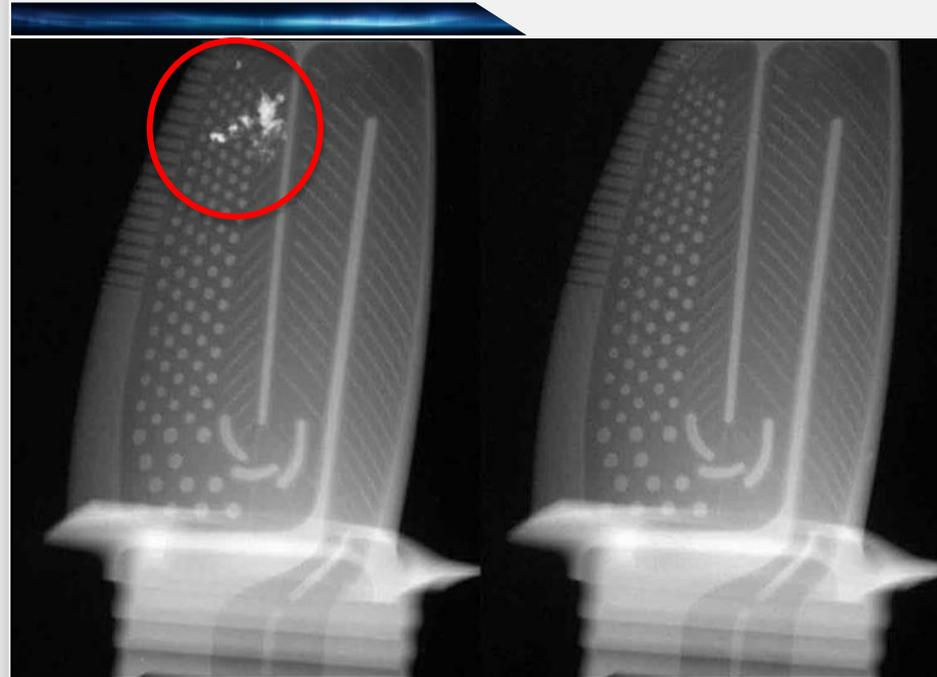
Picture shows two turbine blades exposed to neutron radiography at MNR. The blade on the left shows material from the molding process left in the cooling channels.
