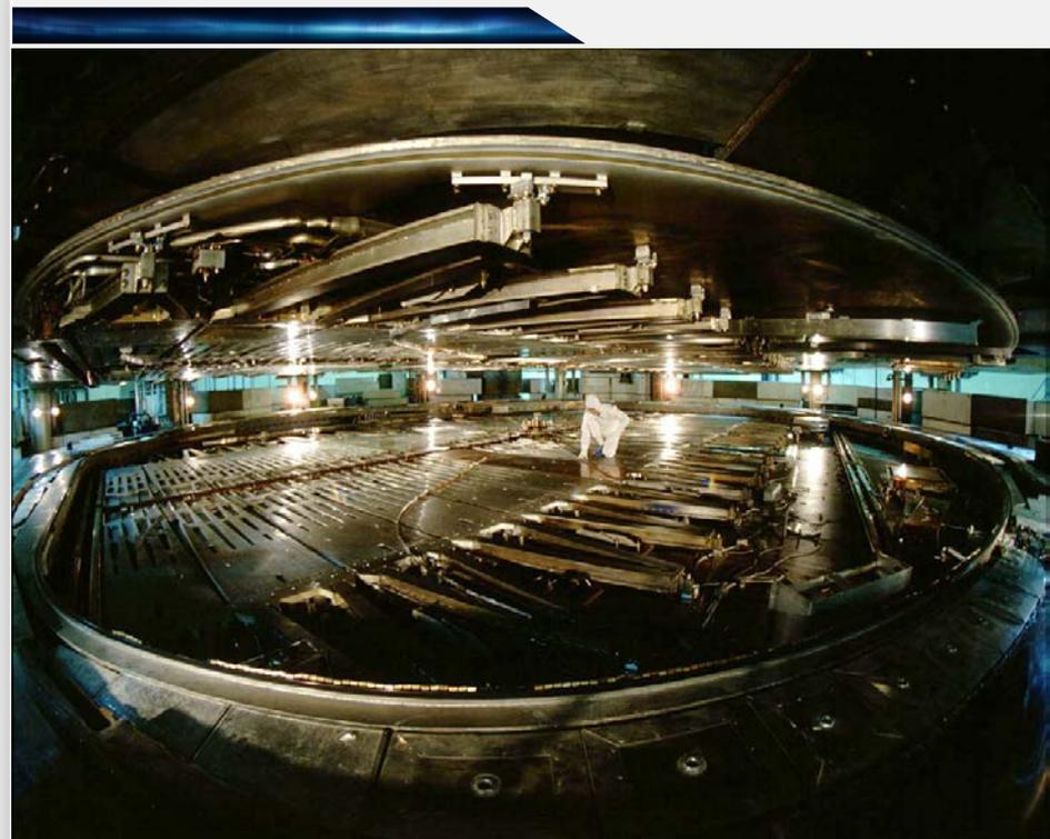
The photo on the right shows the 520 MeV cyclotron tank open.
