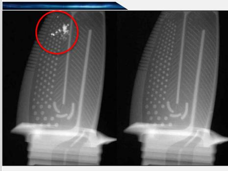
Picture shows two turbine blades exposed to neutron radiography at MNR. The blade on the left shows material from the molding process left in the cooling channels.
