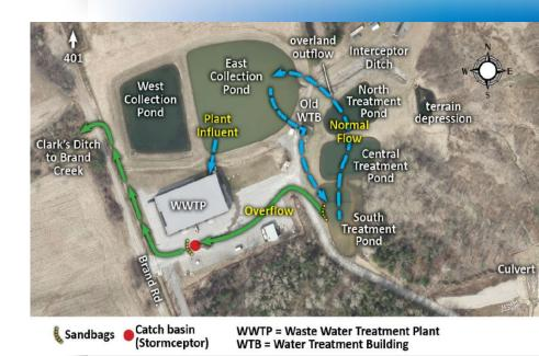
Layout of water management features at the Port Hope LTWMF, and path of June 23, 2017 overflow. (Photo courtesy CNL)
