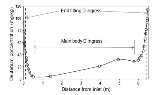
The deuterium concentration increases along the main body of the pressure tube peaking near the outlet end. Approximately 2%–10% of the deuterium generated by the corrosion process is absorbed along the body of the tube.
