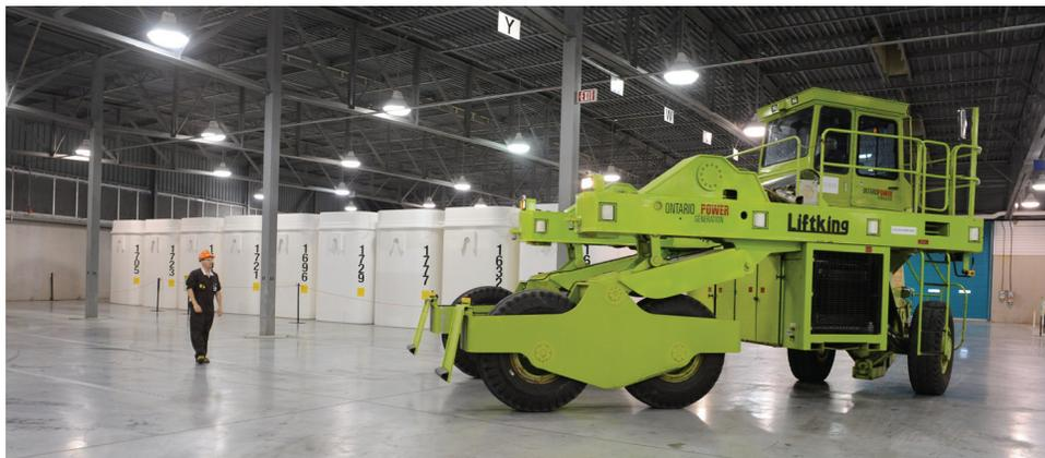
Dry Storage Container transport vehicle at Pickering Waste Management Facility
