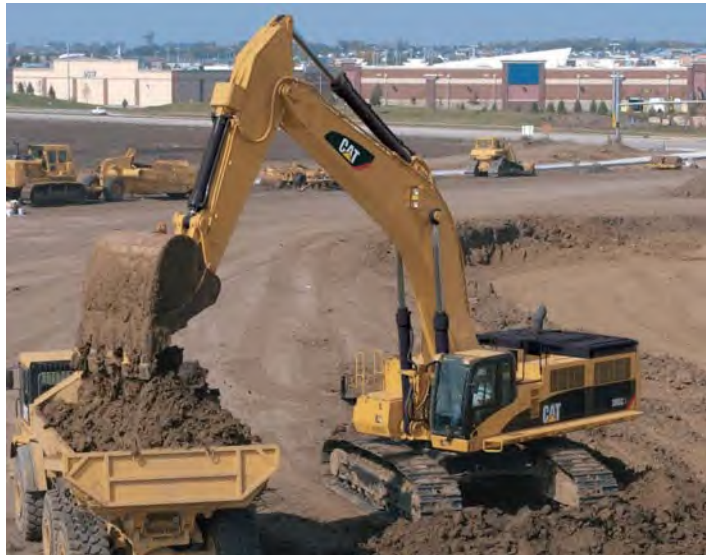
Excavator and Off-Highway Truck (Caterpillar Inc. 2008)
