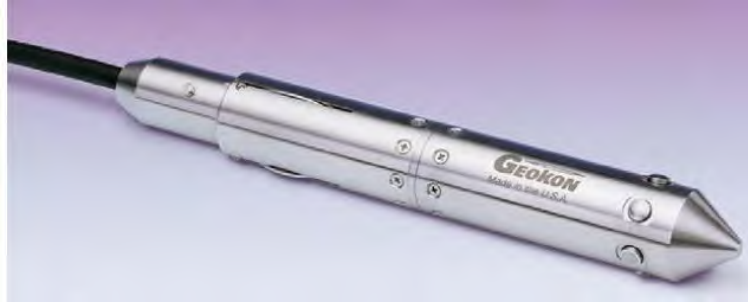
Figure G-2: Photograph of a USBM borehole deformation gauge.
