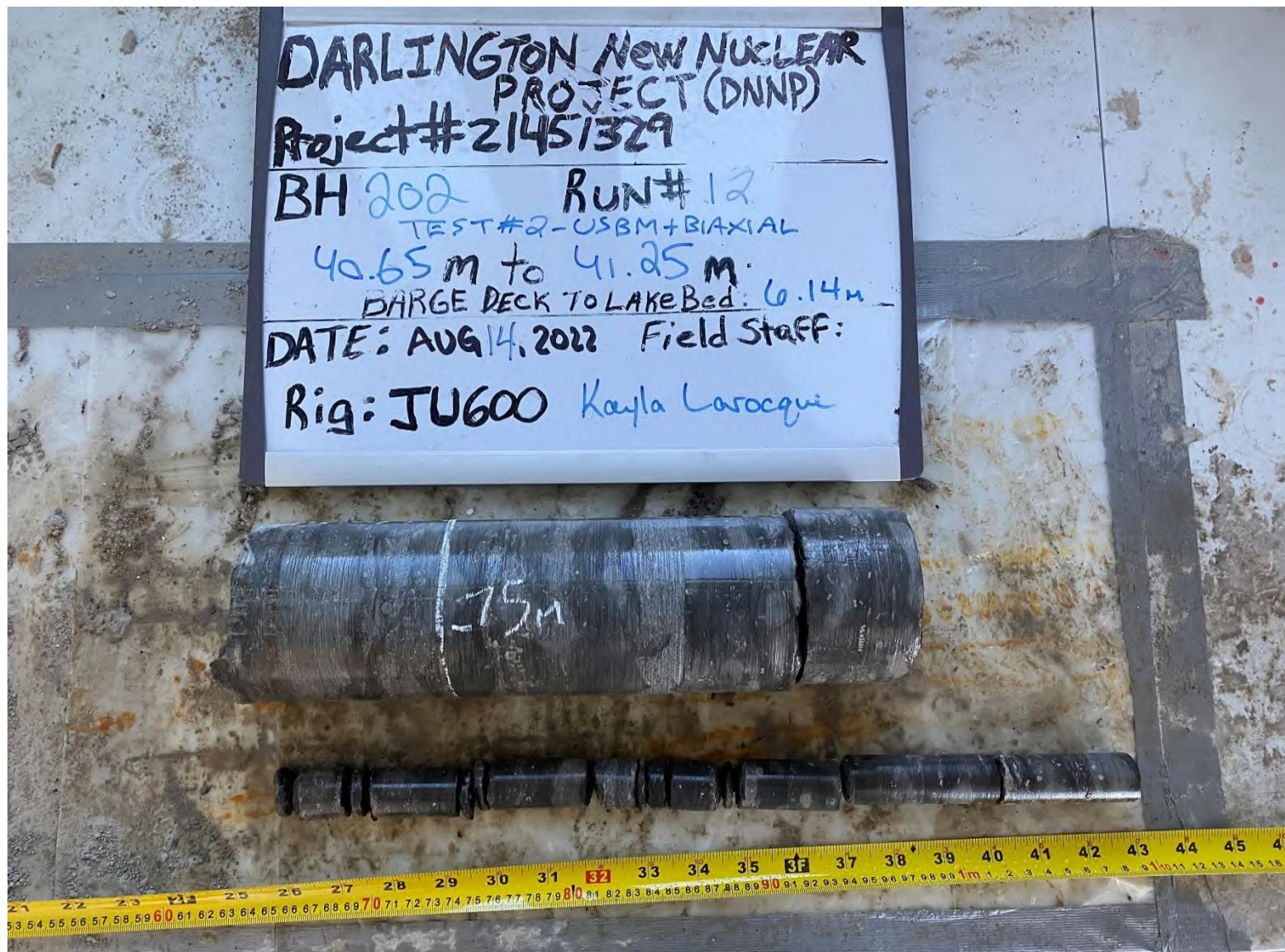
Figure A14: Photograph of retrieved core for Test #2 BH-202-2 (40.65m)
