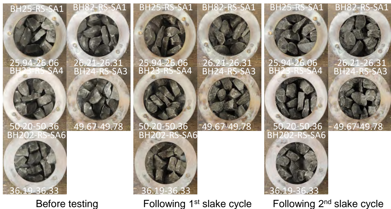
Figure 24: Photographs of slake durability specimen before and after testing.
