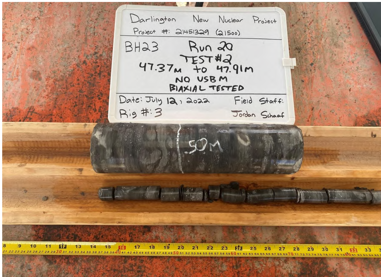
Figure A4: Photograph of retrieved core for Test #2 BH-23-2 (47.40m)
