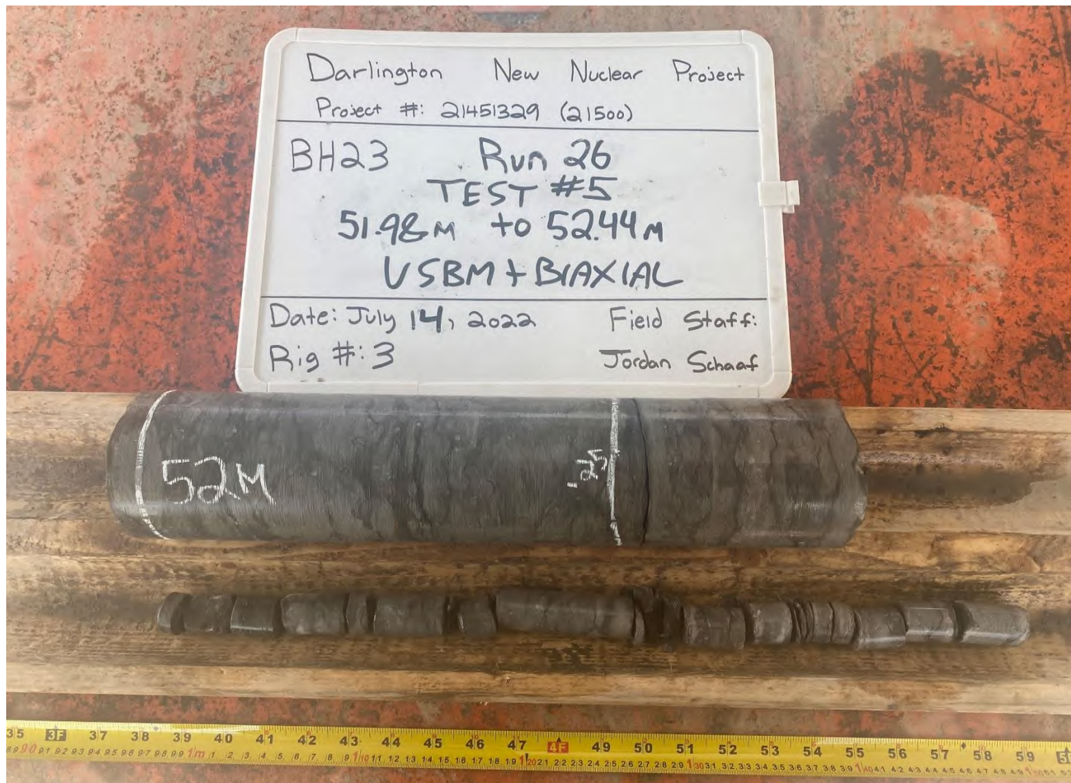
Figure A8: Photograph of retrieved core for Test #5 BH-23-5 (52.00m)
