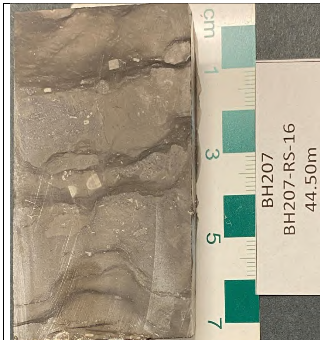
Photograph 1: Sawn rock sample illustrating bioturbation layers of the shale. Field of view is approximately 60 mm across.
