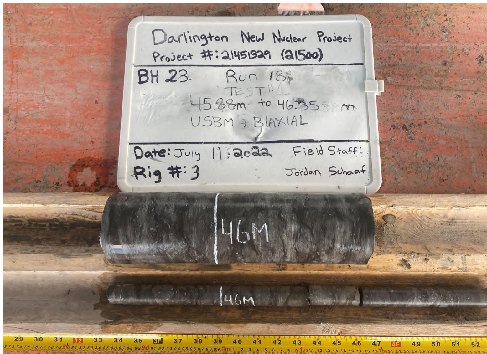
Figure A2: Photograph of retrieved core for Test #1 BH-23-1 (45.88m)
