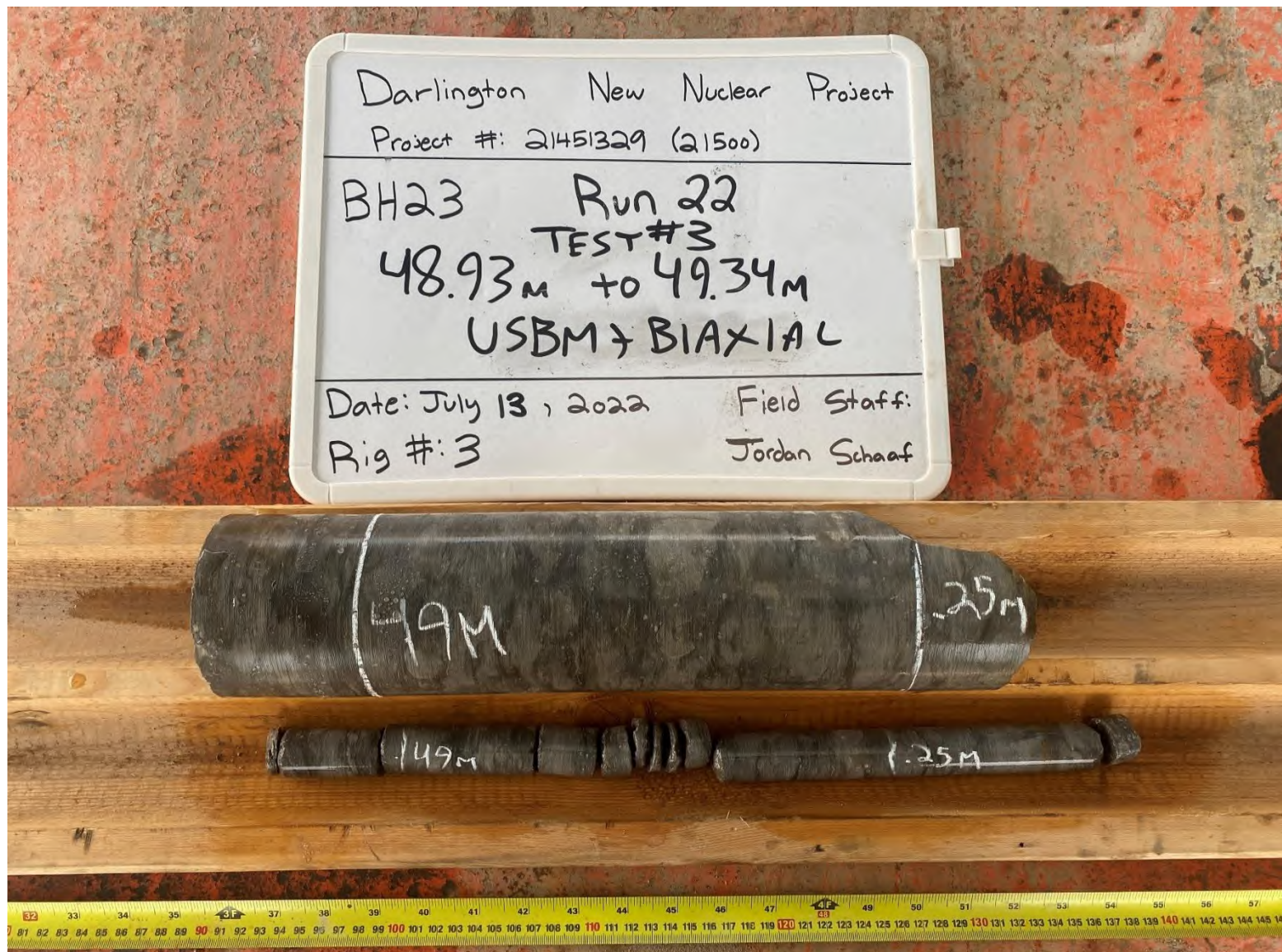
Figure A6: Photograph of retrieved core for Test #3 BH-23-3 (48.90m)
