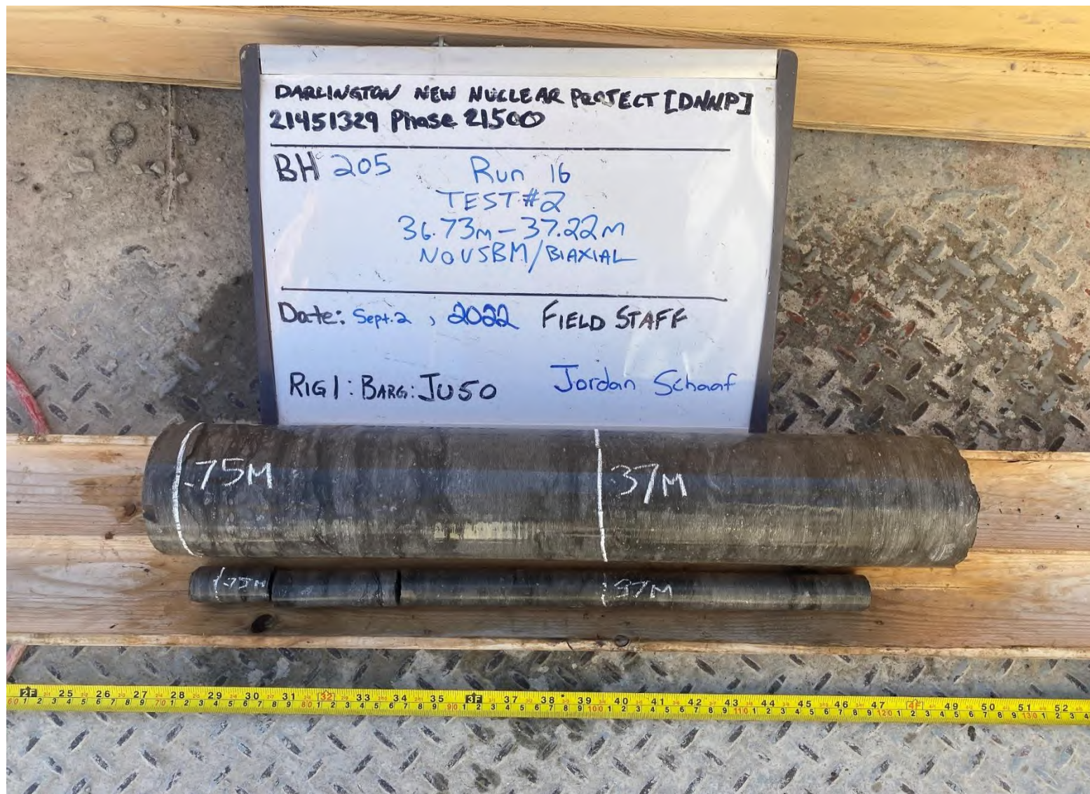
Figure A20: Photograph of retrieved core for Test #2 BH-205-2 (36.73m)
