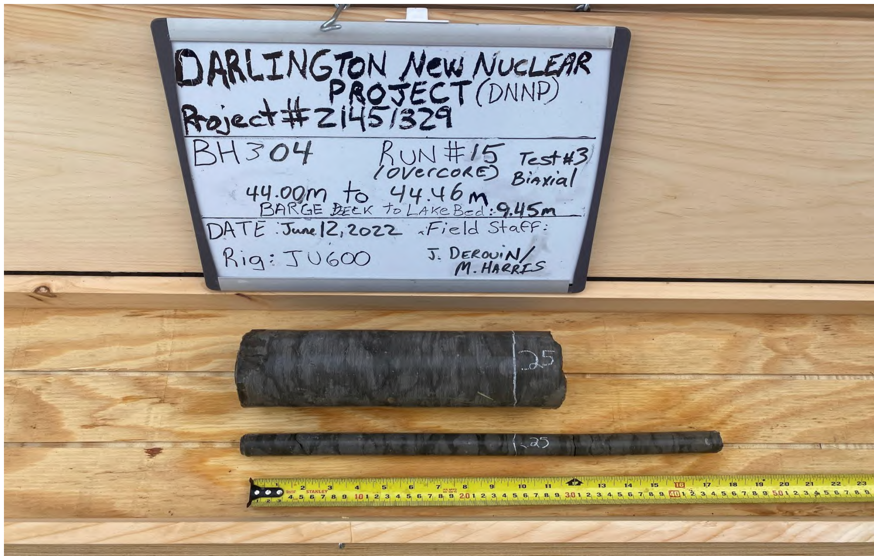
Figure A32: Photograph of retrieved core for Test #3 BH-304-3 (44.00m)
