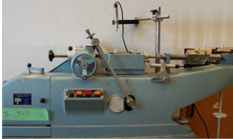
Figure 30: Direct Shear test setup.
