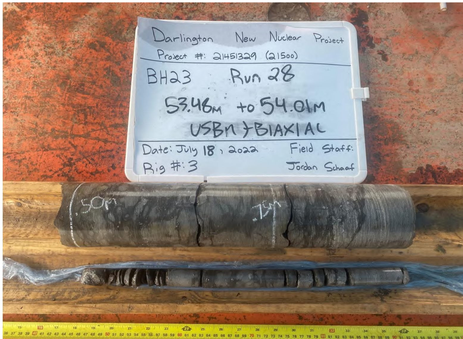
Figure A10: Photograph of retrieved core for Test #6 BH-23-6 (53.50m)
