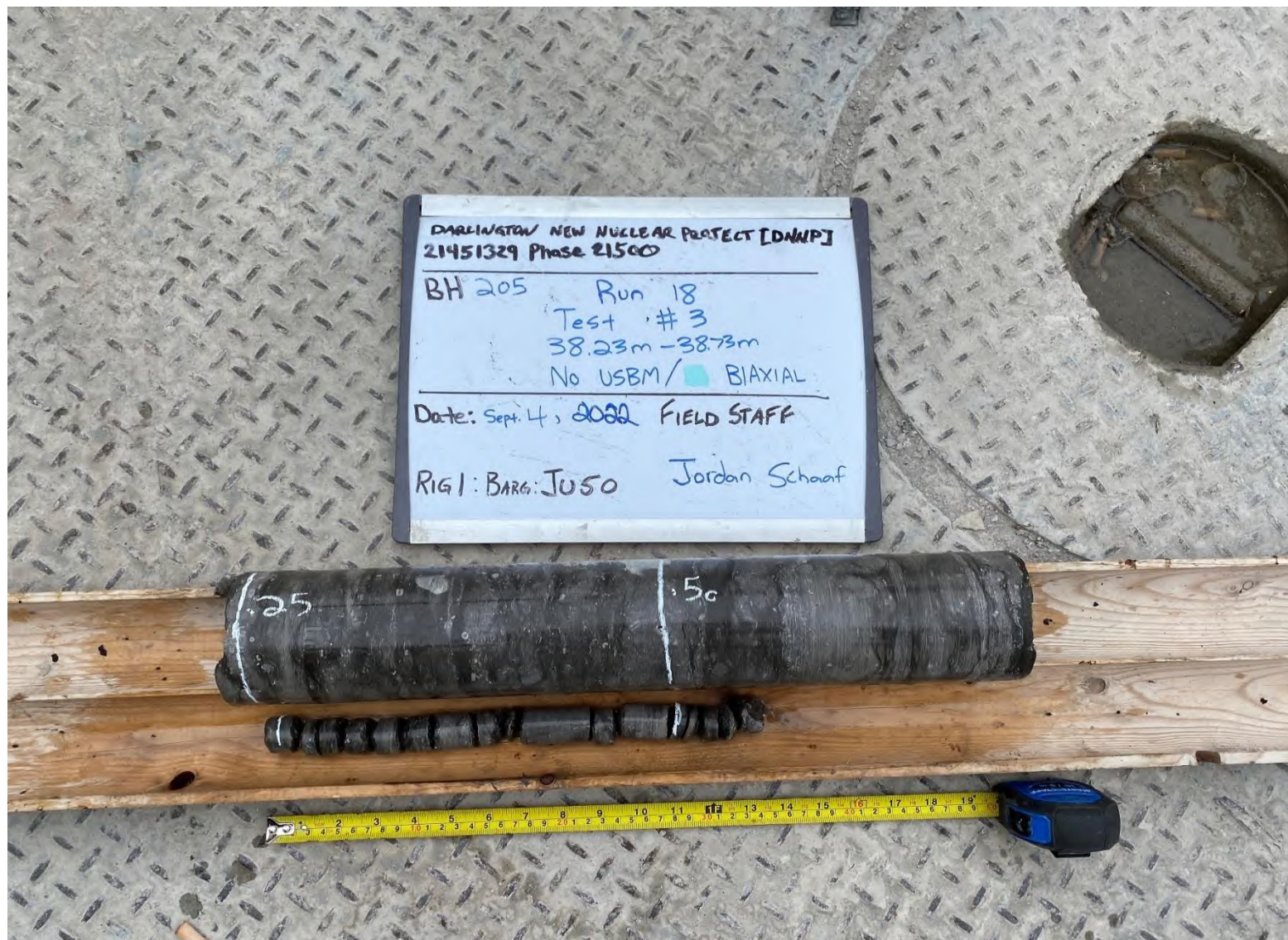
Figure A22: Photograph of retrieved core for Test #3 BH-205-3 (38.20m)
