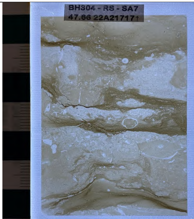
Photograph 2: Thin-section viewed in plane light, no magnification. Field of view is about 45 mm across.
