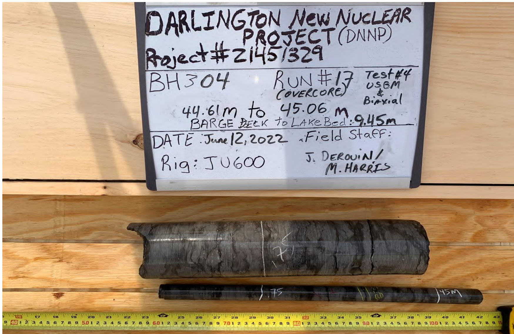
Figure A34: Photograph of retrieved core for Test #4 BH-304-4 (44.60m)
