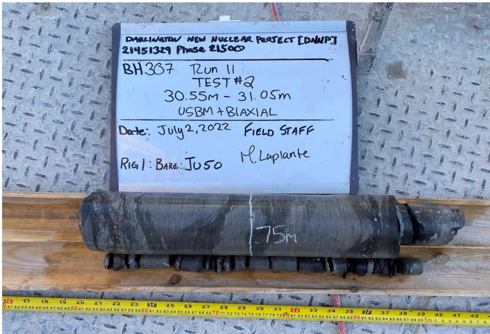
Figure A36: Photograph of retrieved core for Test #2 BH-307-2 (30.60m)
