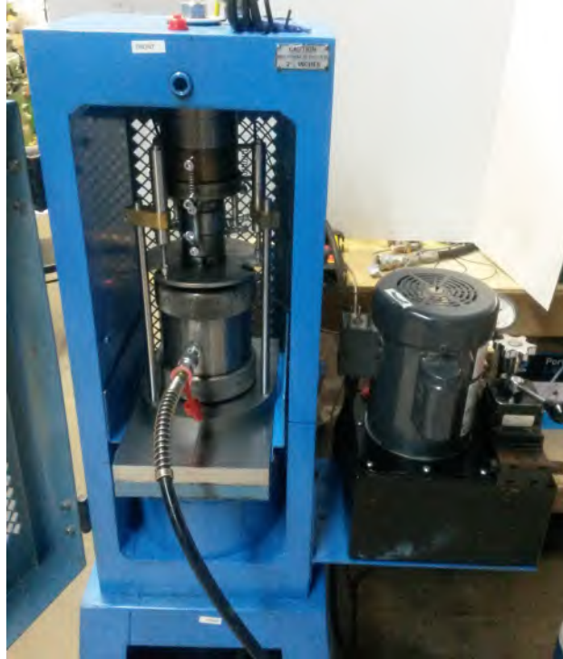
Figure 9: Triaxial test setup, including loading frame and Hoek cell.
