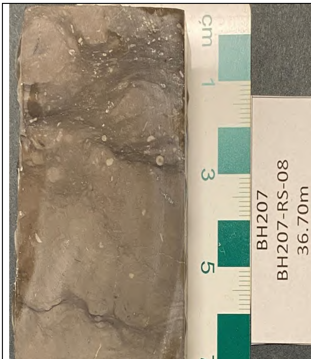
Photograph 1: Sawn rock sample illustrating bioturbation layers of the shale. Field of view is approximately 60 mm across.
