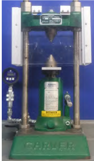
Figure 15: Point load tester equipped with digital pressure gauge.
