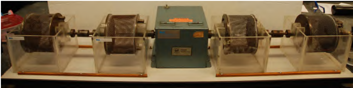
Figure 22: Test setup showing the slake durability apparatus.
