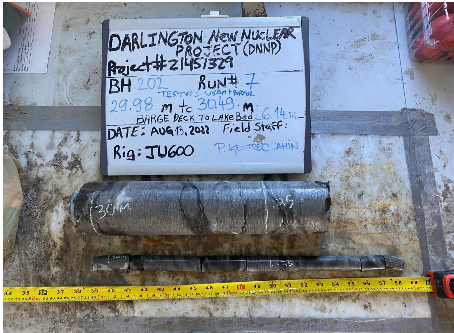
Figure A12: Photograph of retrieved core for Test #1 BH-202-1 (29.98m)
