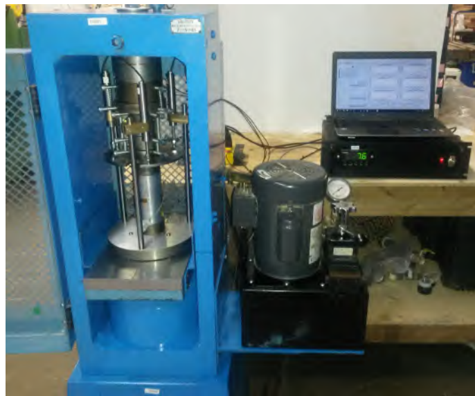
Figure 1: Forney loading frame setup for UCS testing.
