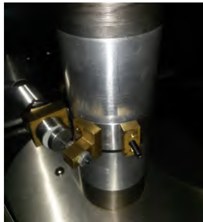
Figure 2: Radial strain sensor comprised of a radial spring and non-contact displacement transducer positioned on the aluminum calibration cylinder.
