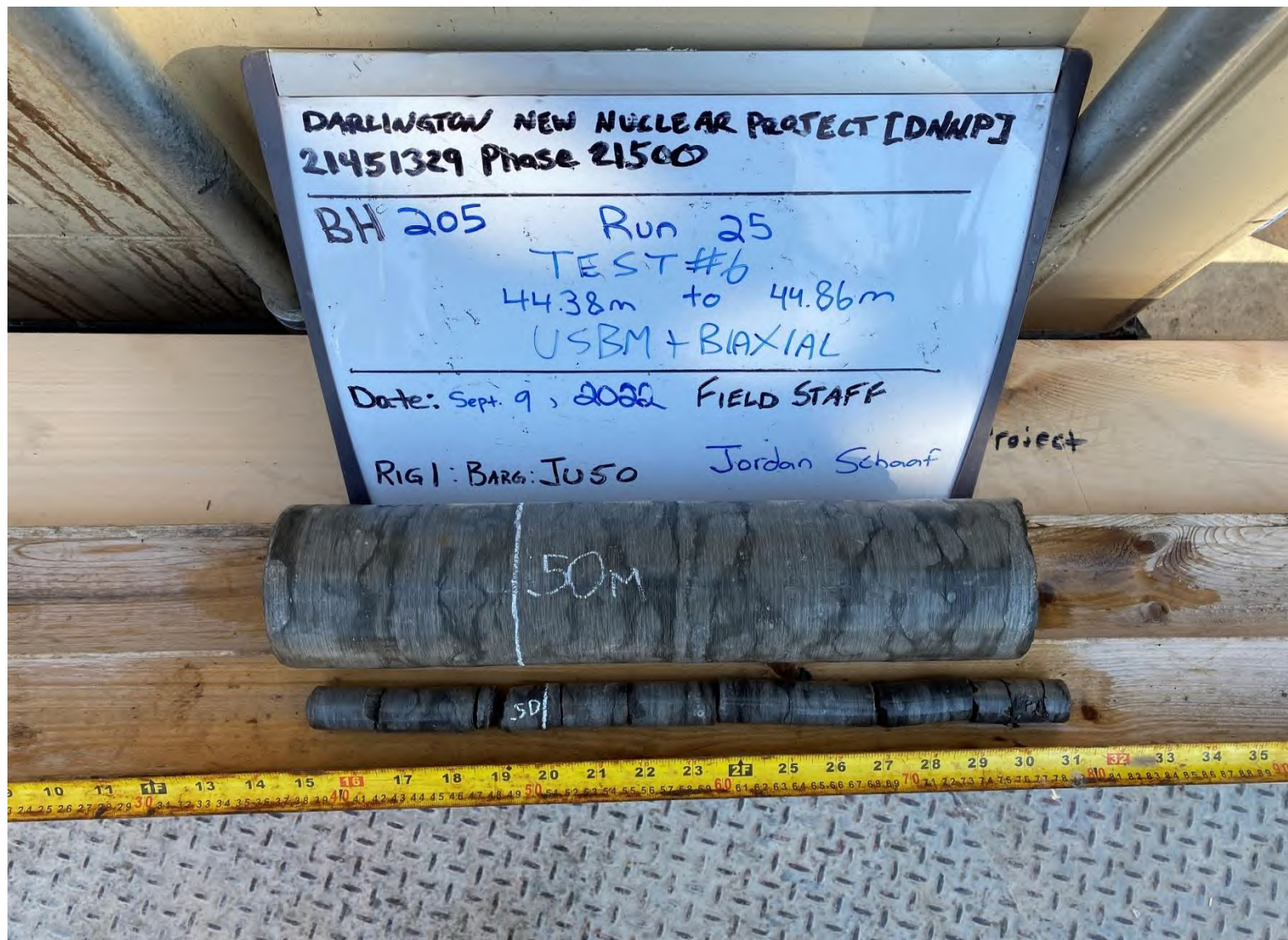
Figure A26: Photograph of retrieved core for Test #6 BH-205-6 (44.86m)
