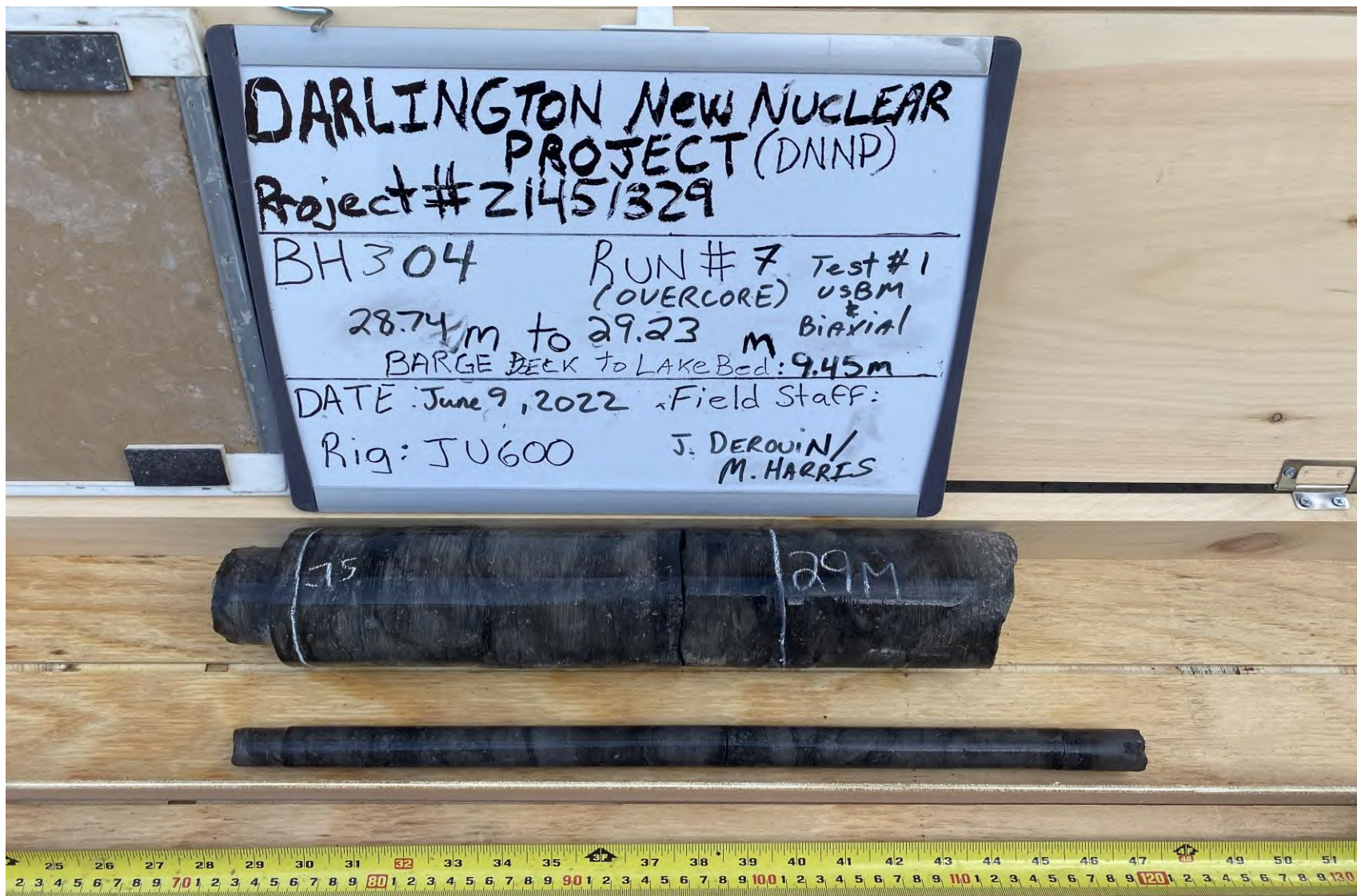
Figure A28: Photograph of retrieved core for Test #1 BH-304-1 (28.70m)
