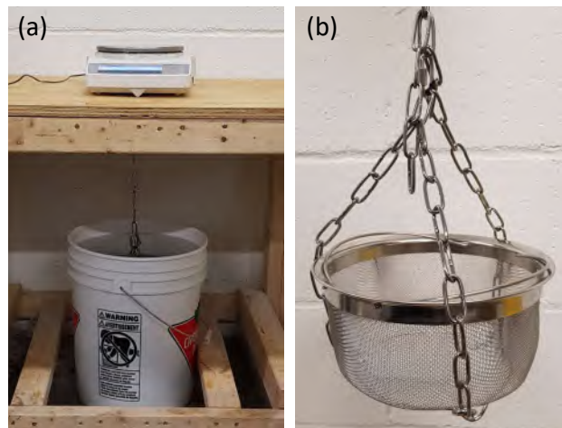
Figure 29: Measuring setup for submerged sample weighing: (a) balance setup and (b) sample basket.
