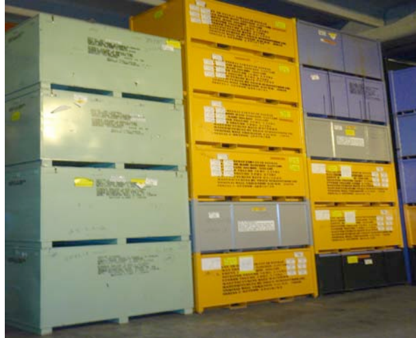
Figure H.1 – OPG low- and intermediate-level waste storage bins at Western Waste Management Facility
