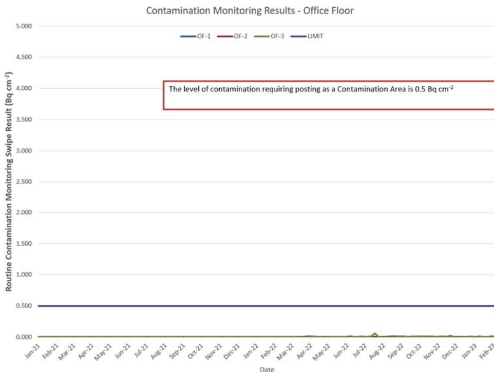
Figure 2.7.2-5 – Contamination monitoring results for the office floor
