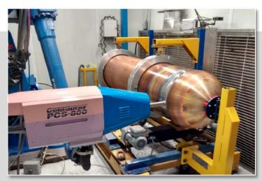
Cold spray copper coating being applied to container lid weld region (courtesy NWMO)
