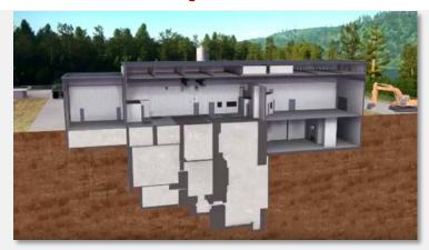
NPD below grade structure containing reactor vessel, system and components will be encased with grout.
