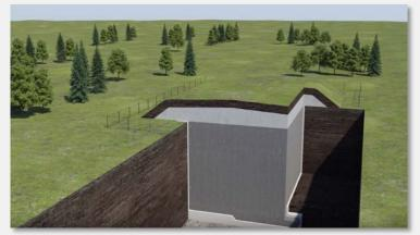
An engineered cover will then be installed over the grouted monolith to prevent intrusion.
