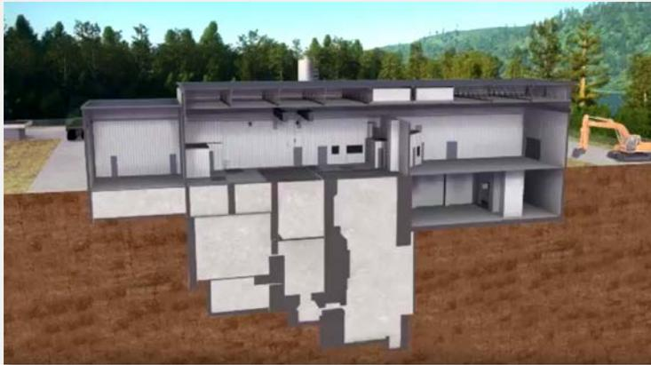
NPD below grade structure containing reactor vessel, system and components will be encased with grout.
