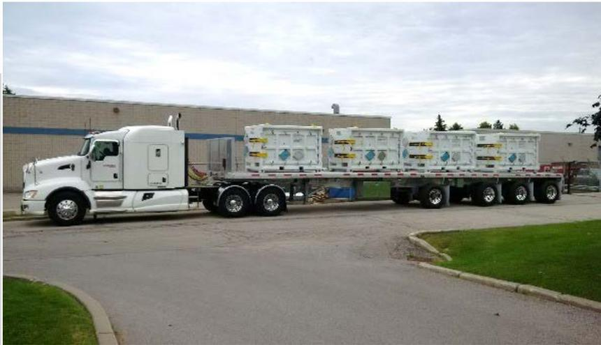
The DSTAR Transportation Package Containing Feeder Tubes
