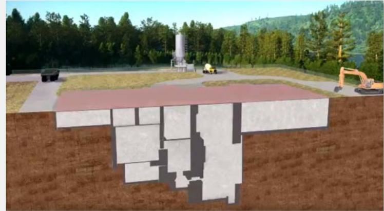
The above ground structures will be demolished and the debris placed in the below grade structure previously occupied by the electrical generating equipment and filled with grout.
