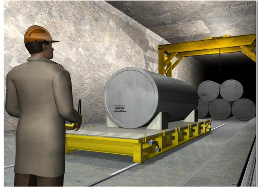
Conceptual emplacement for intermediate-level waste
