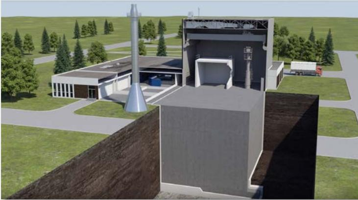
Because it is primarily located low grade the majority of contamination is in the reactor core the entire below grade portion will be filled with grout.
