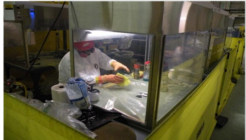
Workers sorting through radioactive waste to divert to volume reduction streams or for free release
