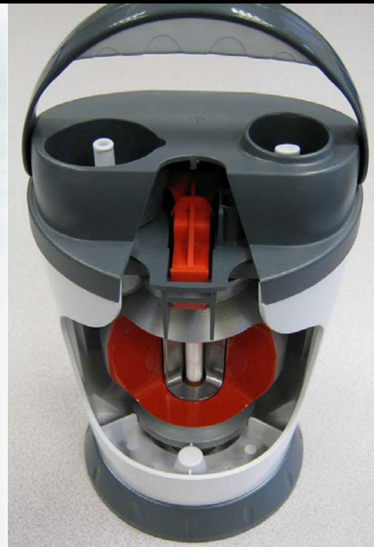
A cutaway model of a technetium generator. The molybdenum/alumina sample is placed in the centre of the device, surrounded by shielding (painted red in this case).
