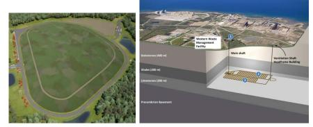
Design picture of proposed near surface disposal facility, which will be located at the current site of Chalk River Laboratories, Ontario - Picture courtesy of CNL
