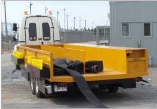
Hose trailer for emergency water make-up
