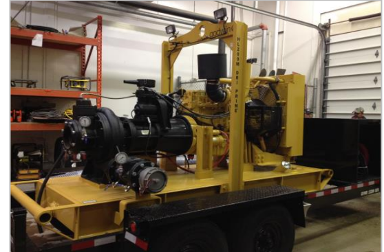
Emergency water supply pump to further strengthen emergency preparedness
